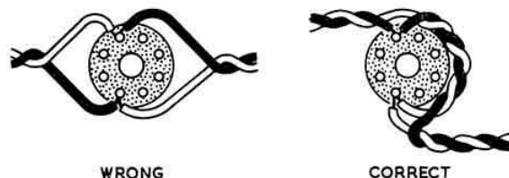
Fig. 6. How incorrect heater wiring can leave a loop under the valve holder. The correct method is shown on the right.
