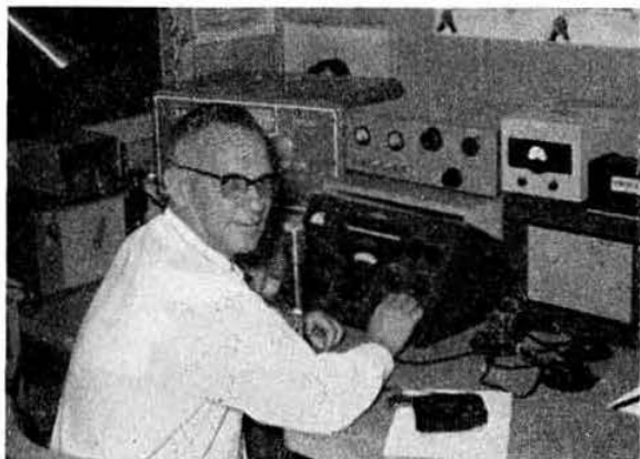
ZS5JY keeps a sked with his wife ZS5PI during a visit to KH6DLF. The two boxes above the receiver contain the three 4CX-250As used in the kilowatt p.a.
